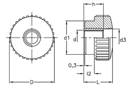
$$\begin{array}{ll} D & = 15 \\ d1 & = 11 \\ d3 & = 6 \\ d \ 6H = M4 \\ h & = 10 \\ L & = 11.0 \end{array}$$
